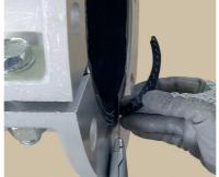
5. Cut off excess hose protruding past the coupling face
