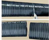
2. Cut the hose with a sharp cutting tool up to the steel helix wire
