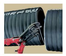
3. Cut the steel helix wire. The wire must not protrude past the end of the hose
